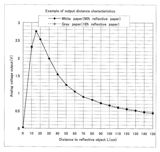
7-2 GP2Y0A02YK0F Example of output distance characteristics with the inverse of distance
